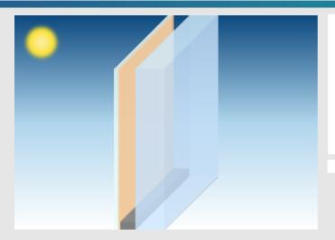
PLANICLEAR (4 mm) Pane 1 PLANITHERM XN Cavity 1 ARGON (90%) / AIR (10%) / 14 mm Pane 2 CF60-3 5445 (27 mm)
